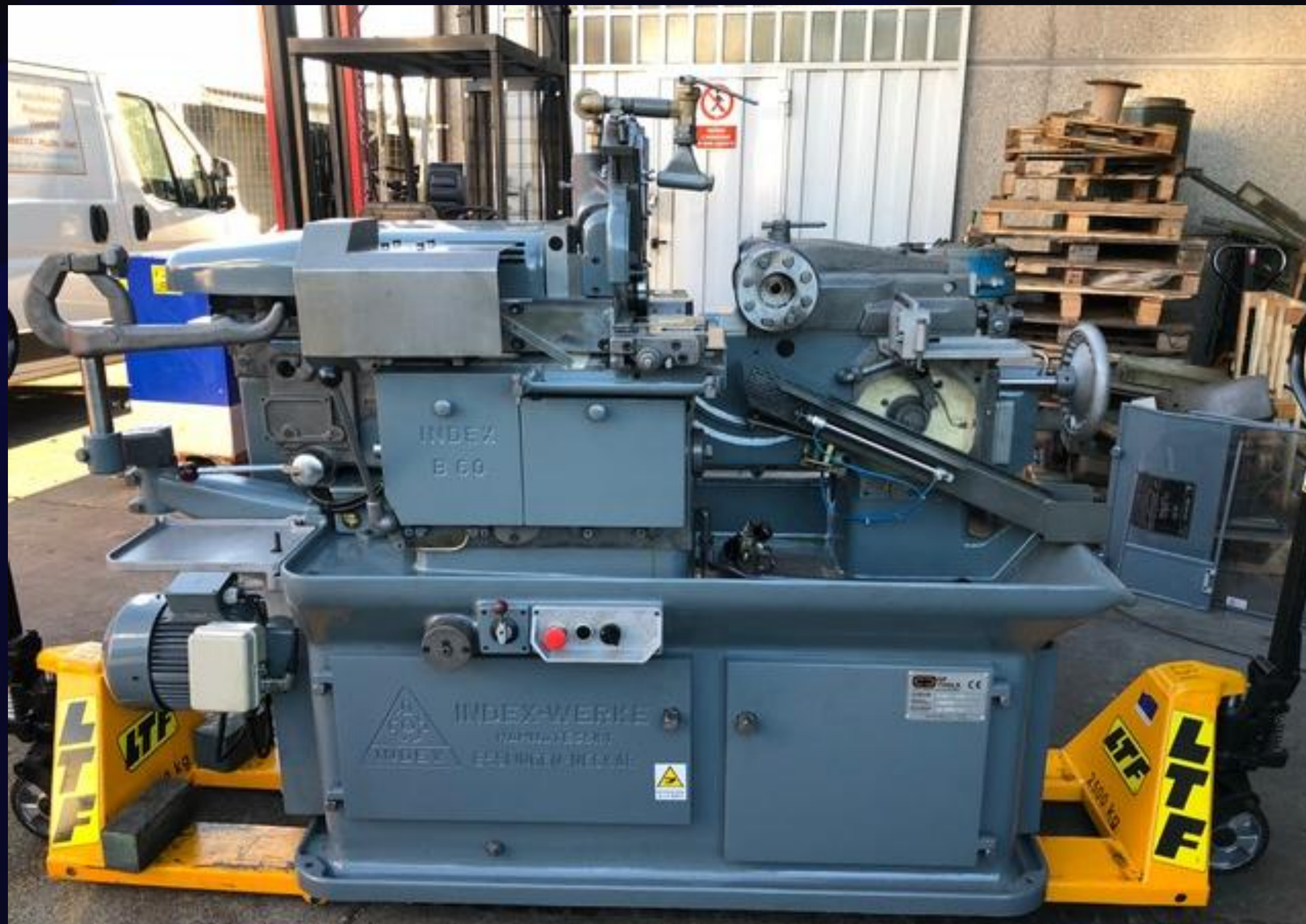
Index B60 Cam driven lathe, fully automatic
