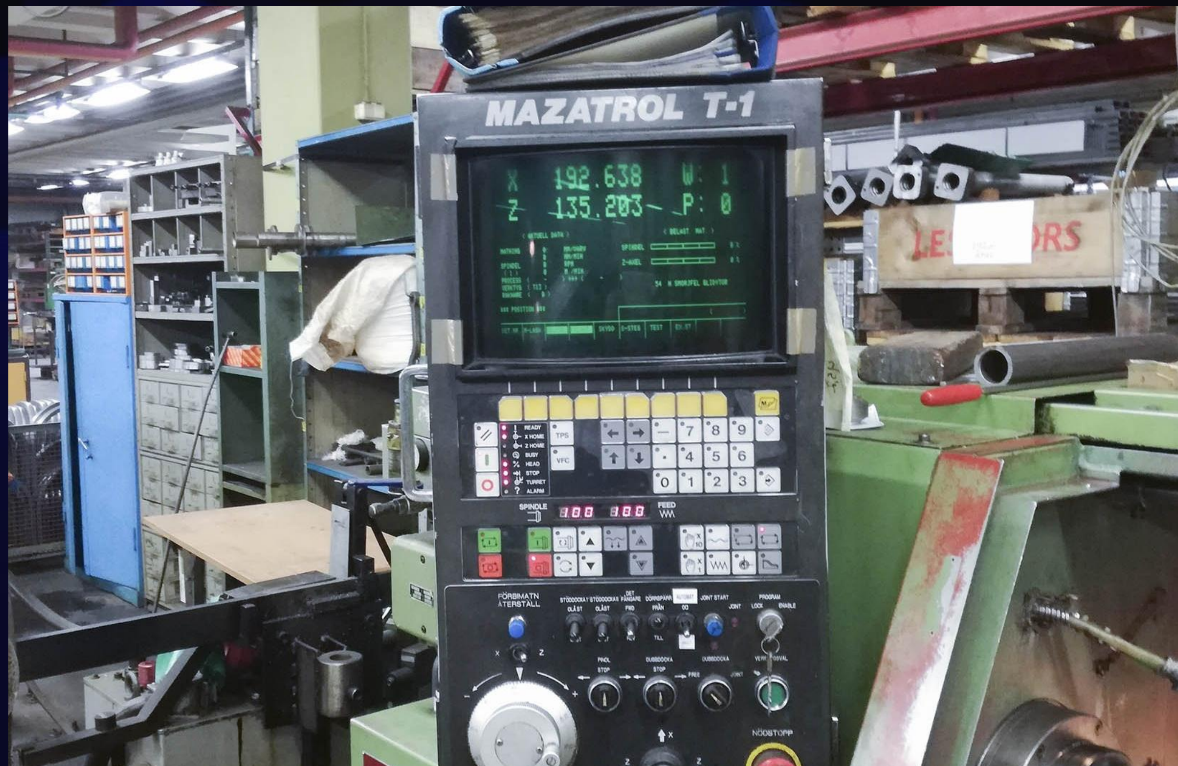
Mazak Lathe running Mazatrol T-1
